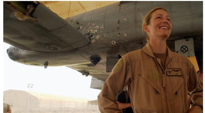
A great example of redundant systems is the A-10 Warthog, a plane used by the US Air Force for almost 50 years. The aircraft's purpose was close combat support and needed to work even when taking enemy fire. Its entire design was built on redundant systems. If one system failed, another kicked in.
